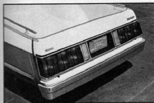
Stock Fairmont taillight / license assembly graces the broad tailgate which is steel-reinforced.
